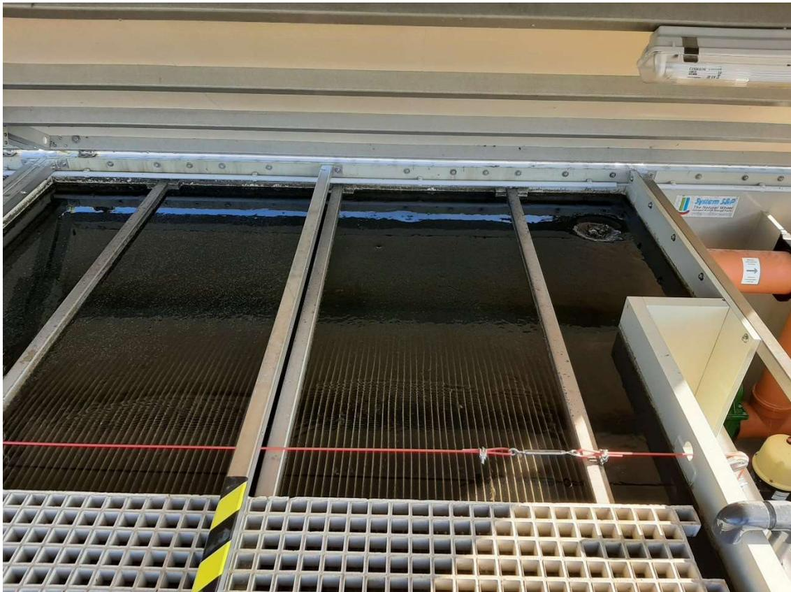
The submerged discs are clearly recognizable, which allows the continuity of the process with easy access at the same time.
